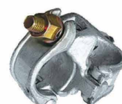
WD-0001P GERMAN TYPE DOUBLE COUPLER 76mmX48.3mm 1.10 KGS
