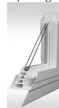
Flush frame window: Flush frame windows have the fin at the exterior surface of the window and seal to a flat exterior surface like stucco.
