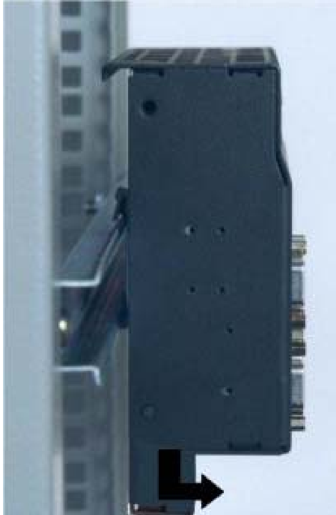
Figure 28. Removing from the Standard Rail
