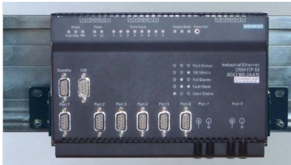
Figure 29: Installation on the S7-300 Rail
