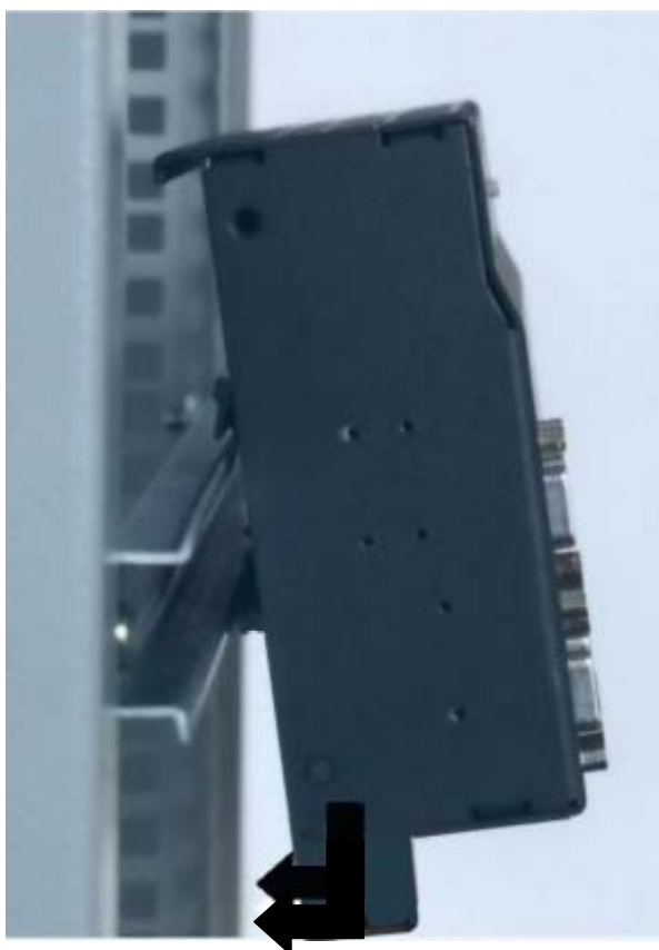
Figure 27: Installing the OSM on a DIN Standard Rail
