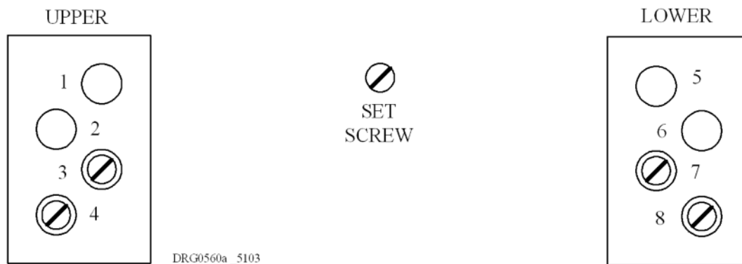
Figure 2-1 Chassis mechanical coding block configurations
