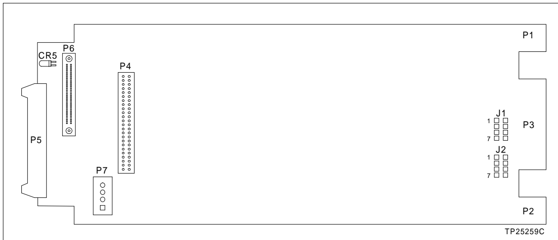
Figure 3-2. IMMPI01 Jumper Locations
