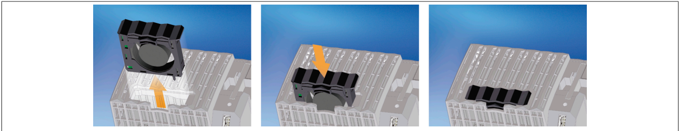
Figure 12: X20 CPUs - Tool-free fan replacement
