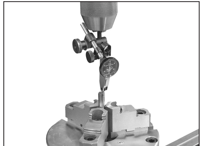
Figure 11. Horizontally aligning the chuck.
