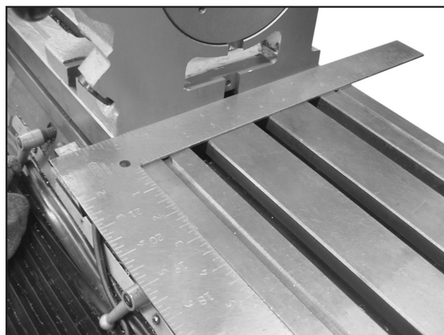
Figure 9. Using a precision square to align with X-axis.
