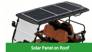
Solar Panel on Roof
