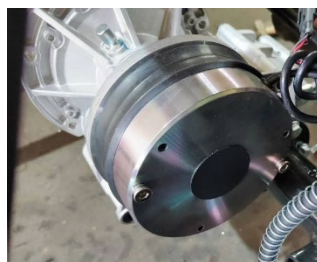
1) Electromagnetic parking brake(EPB)
