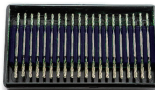
FLE040 Grit: #120/140 Shank dia.: 3.175mm Head dia.: 1.6mm and 2.1mm Total length: 46mm Application: jade, glass and other hard brittle materials hole processing
