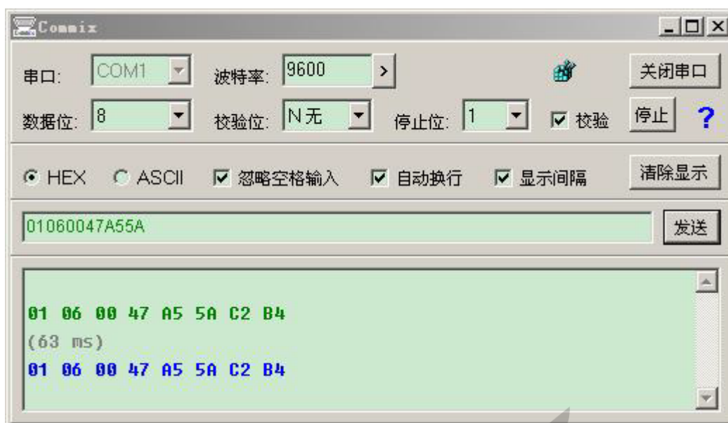
Figure 4-1 Total Zeroing Frame Structure
