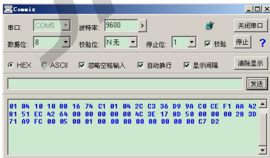
Figure 6-5 Example of Serial Port Debugging Assistant Listening
