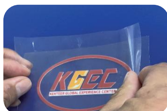
5 Use Transfer Tape To Position The Pattern
