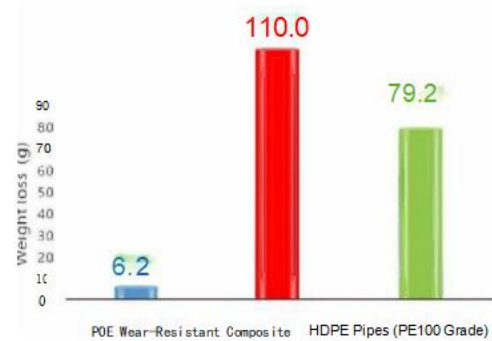
Evaluation of wear resistance in pipe form
