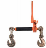
Item No.: BTFHLB09 Material: Forged Steel Chain Size: G70 & G80 1/4" - 5/16" W.L.L.: 2,200lbs
