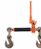
Item No.: BTFHLB12 Material: Forged Steel Chain Size: G70 & G80 1/2" - 5/8" W.L.L.: 18,000lbs
