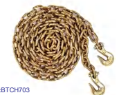
Item No.:BTCH703 Material:Carbon Steel Chain size:1/2" Safety factor:4:1 W.L.L.:11300lbs Assembly BS:45200lbs
