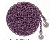
Item No.: BTCH104 Material: Alloy Steel Chain size: 5/8" Safety factor: 4:1 W.L.L.: 22,600lbs Assembly BS: 90,400lbs
