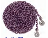
Item No.: BTCH101 Material: Alloy Steel Chain size: 5/16" Safety factor: 4:1 W.L.L.: 5,700lbs Assembly BS: 22,800lbs
