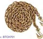
Item No.: BTCH701 Material: Carbon Steel Chain size: 5/16" Safety factor: 4:1 W.L.L.: 4,700lbs Assembly BS: 18,800lbs
