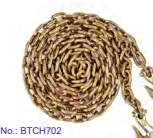
Item No.: BTCH702 Material: Carbon Steel Chain size: 3/8" Safety factor: 4:1 W.L.L.: 6,600lbs Assembly BS: 26,400lbs
