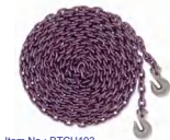
Item No.: BTCH103 Material: Alloy Steel Chain size: 1/2" Safety factor: 4:1 W.L.L.: 15,000lbs Assembly BS: 60,000lbs
