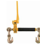
Item No.: BTFHLB03 Material: Forged Steel Chain Size: G70 & G80 3/8" or 1/2" W.L.L.: 12,000lbs
