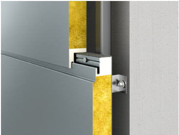
Interlocking with Framing
