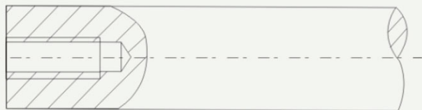
COAXIAL HOLES DRILLED AND TAPPED
