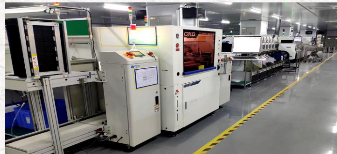
SMT production is equipped with Fuji NXTIII high-speed machine. Supports smallest 01005 components.
