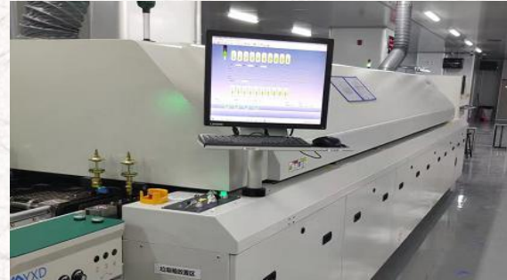
Configured as Jintuo ten temperature zone reflow furnace.
