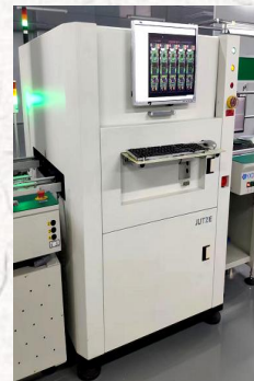
SPI/AOI: Solder paste thickness detector and automatic optical detector
