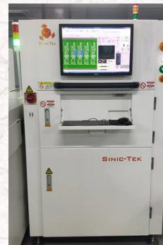
SPI/AOI: Solder paste thickness detector and automatic optical detector
