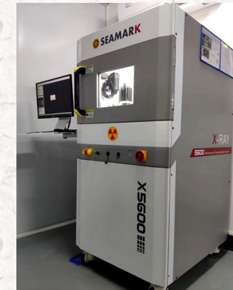
X-RAY equipped for the first article inspection and daily detection and analysis of BGA soldering quality.
